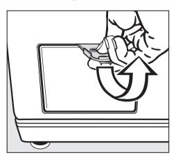
■ Use it to open the access flap and drain the water as described in the "Cleaning the fluff filter and pump" section of "Cleaning and care".
